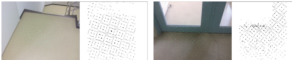
Fig. 7. (Color online) Example of images were incorrectly detected by illuminance of point pattern.
