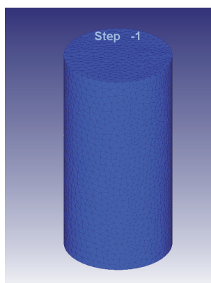
Fig. 1. (Color online) Mesh distribution for the aluminum rod.
