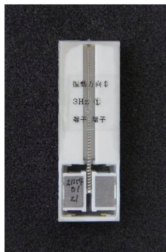
Fig. 16. (Color online) Shape of the sensor with 3 Hz resonance frequency.
