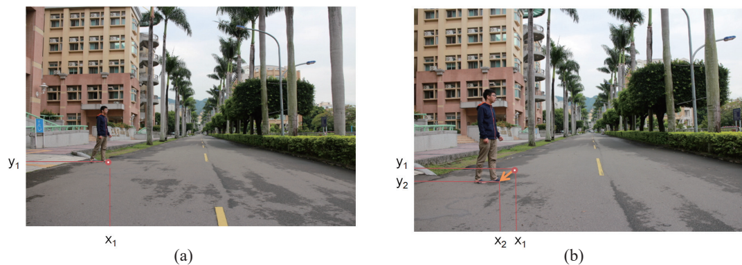
Fig. 3. (Color online) (a) Coordinate of a standing pedestrian in image I(t) . (b) Coordinate of a standing pedestrian in image I(t+1) .
