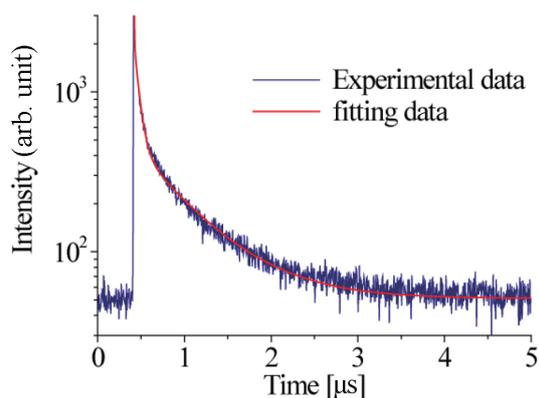
Fig. 5. (Color online) Pulsed-X-ray-induced scintillation decay time profile of the CsSrCl<sub>3</sub>:Ce crystal.
