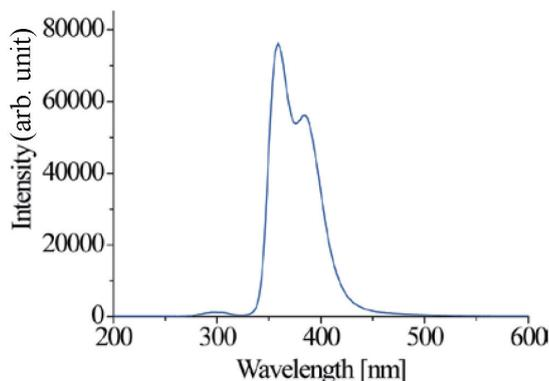
Fig. 4. (Color online) X-ray-induced scintillation spectrum of the  $CsSrCl_3:Ce$  crystal.
