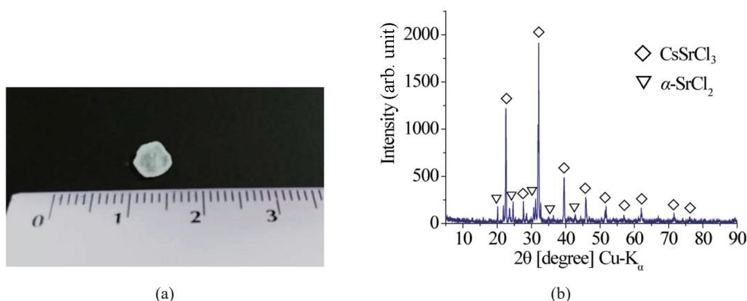
Fig. 1. (Color online) (a) An as-grown  $\text{CsSrCl}_3\text{:Ce}$  crystal and (b) XRD patterns of the crystal.
