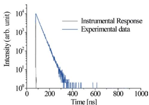
Fig. 3. (Color online) Photoluminescence decay time profile of the  $CsSrCl_3:Ce$  crystal. ( $\lambda_{ex} = 320$  nm,  $\lambda_{em} = 365$  nm)
