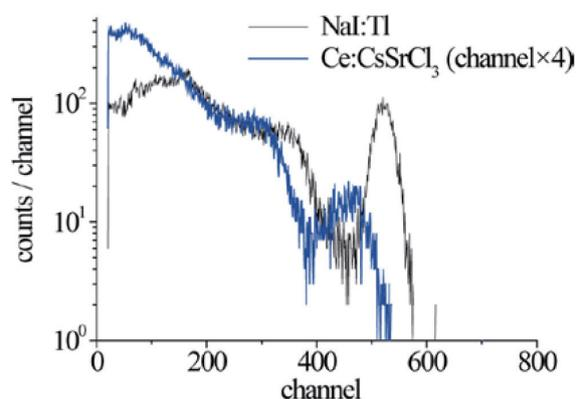
Fig. 6. (Color online) <sup>137</sup>Cs-gamma-ray-induced pulse height spectra for CsSrCl<sub>3</sub>:Ce and the NaI:Tl commercial scintillator.
