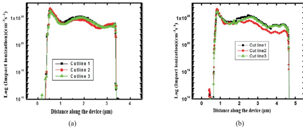
Fig. 3. (Color online) Surface impact ionization distributions of proposed (a) 80 and (b) 100 V NLD MOS unit cells.
