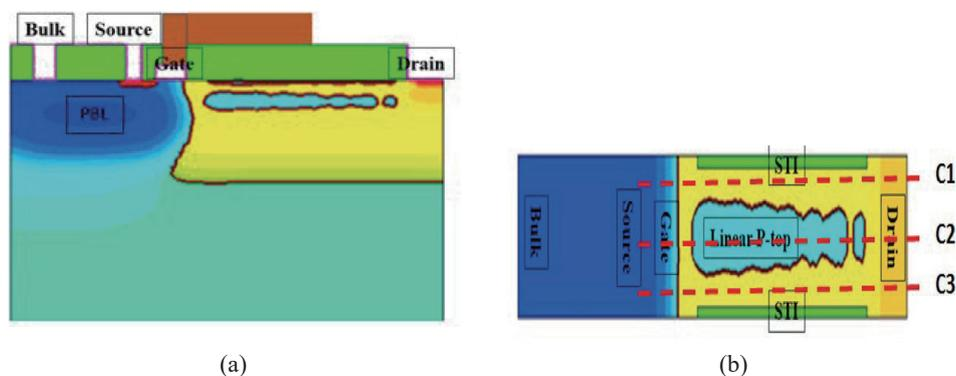
Fig. 2. (Color online) Proposed low-side structure in (a) front and (b) top views.
