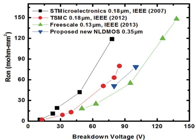
Fig. 6. (Color online) Comparison of benchmark off-state breakdown vs on-state resistance ( $R_{on}$ ) for different technologies.
