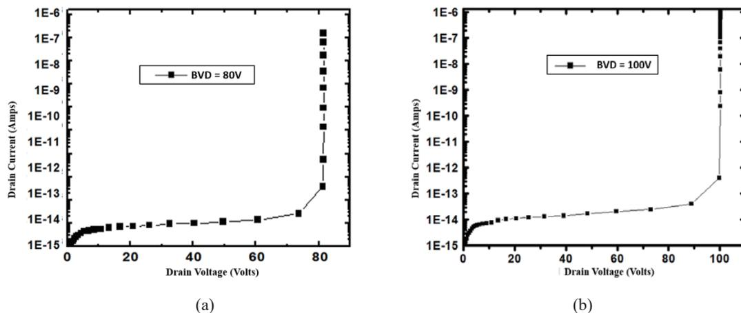
Fig. 4. Breakdown curves for proposed (a) 80 and (b) 100 V NLD MOS unit cells.
