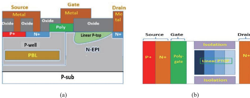
Fig. 1. (Color online) Schematic view of low-side NLDMOS structure with side isolations in (a) front and (b) top views.
