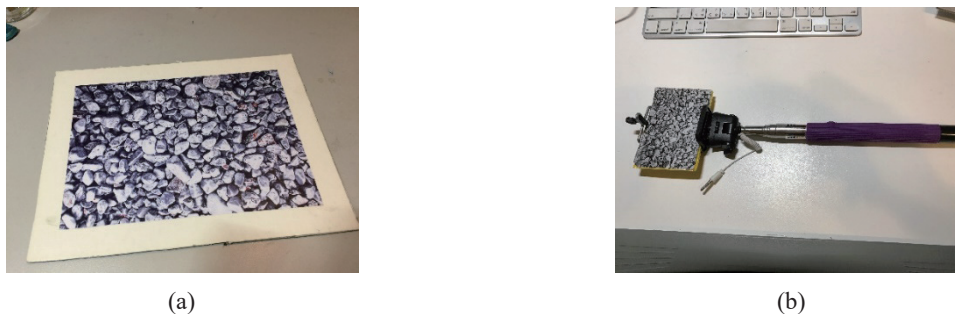
Fig. 2. (Color online) Two image targets that are used to define our (a) workplace and (b) AR Pen.
