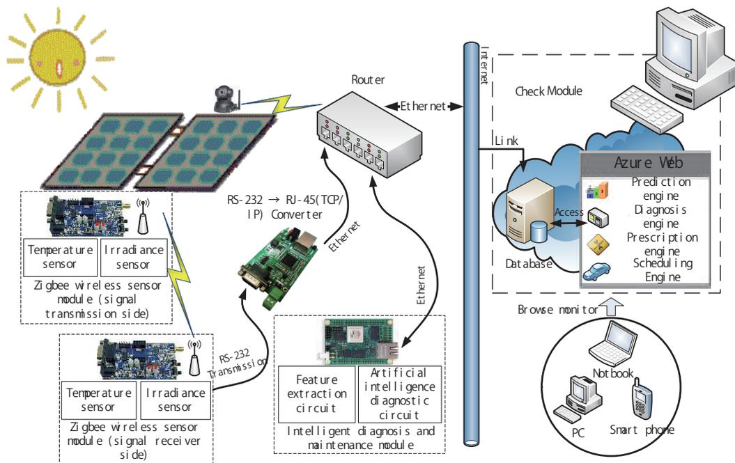
Fig. 1. (Color online) Architecture of maintenance scheduling for solar-energy-generating system.
