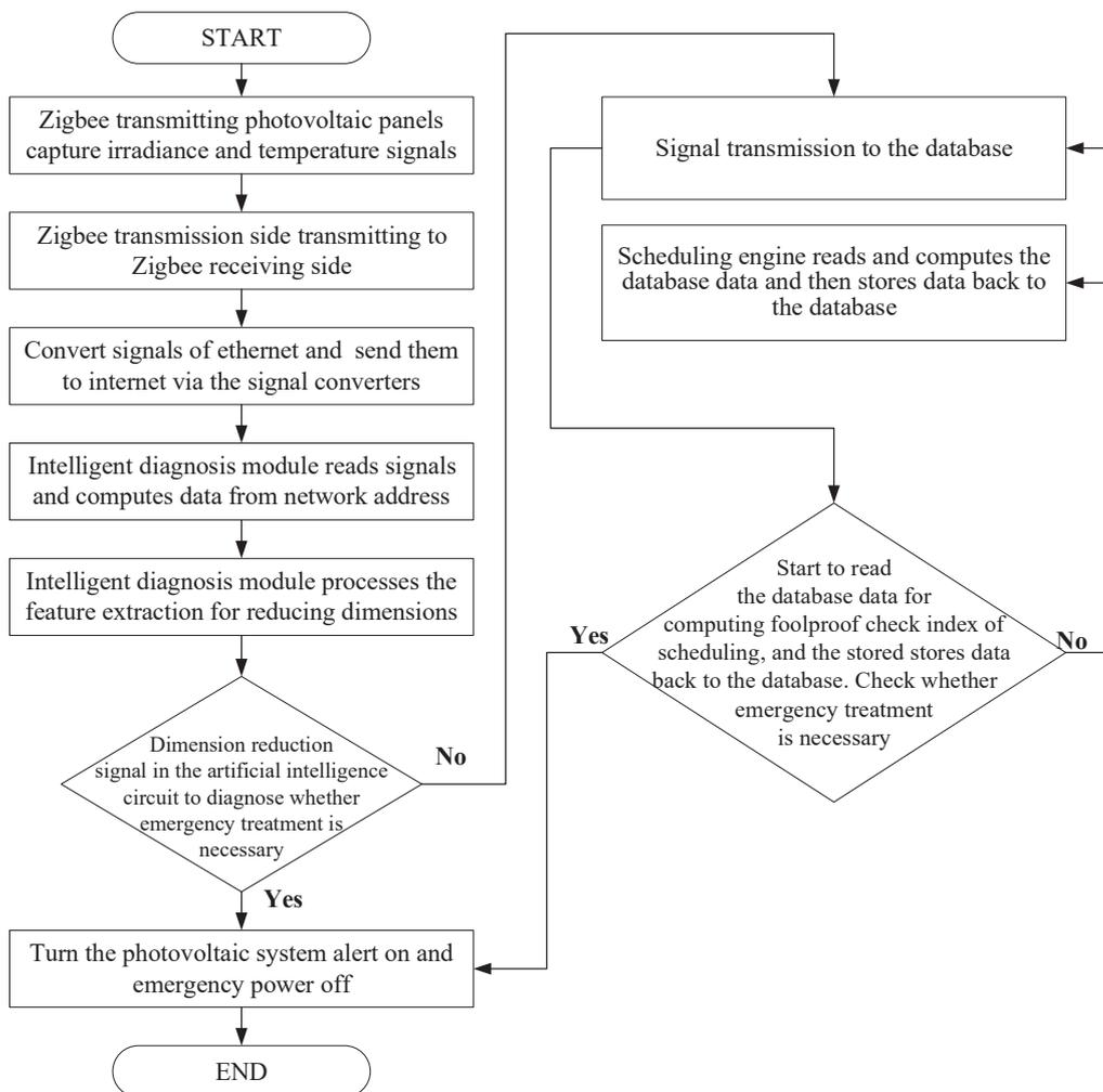
Fig. 2. Flowchart of maintenance scheduling for solar-energy-generating system.
