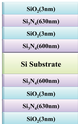
Fig. 1. (Color online) Schematic diagram of the multilayer (consisting of \text{Si}_3\text{N}_4 and \text{SiO}_2 ) antireflection coating on Si substrate. The thicknesses of the \text{SiO}_2 and \text{Si}_3\text{N}_4 layers were optimized using the Essential Macleod program.
