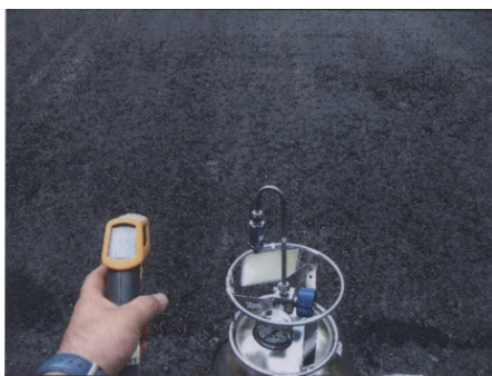
Fig. 3. (Color online) In situ temperature measurements and VOCs detected.
