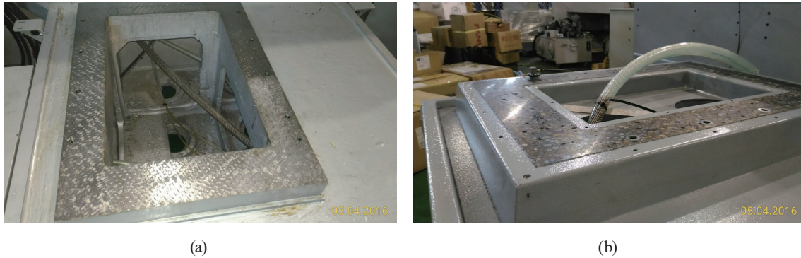
Fig. 3. (Color online) (a) Base of the grinder is cast with cast iron. (b) Base of the grinder is cast with mineral resin.
