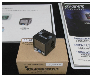
Fig. 7. (Color online) Precise differential pressure sensor module (30 mm cube), Yamamoto Electric Works.
