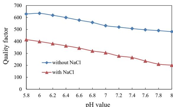
Fig. 4. (Color online)  $Q$  value of a 0.05 M PB solution with and without added NaCl.
