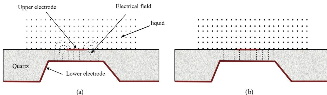
Fig. 3. (Color online) Schematic illustration of the electric field distribution of the QCM with an inverted-mesa structure: (a) in a nonconductive liquid and (b) in a perfectly conductive liquid.
