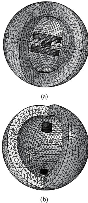
Fig. 2. FEA simulation model of diamagnetic levitation structure: (a) calculation model of diamagnetic force and (b) calculation model of magnetic force.
