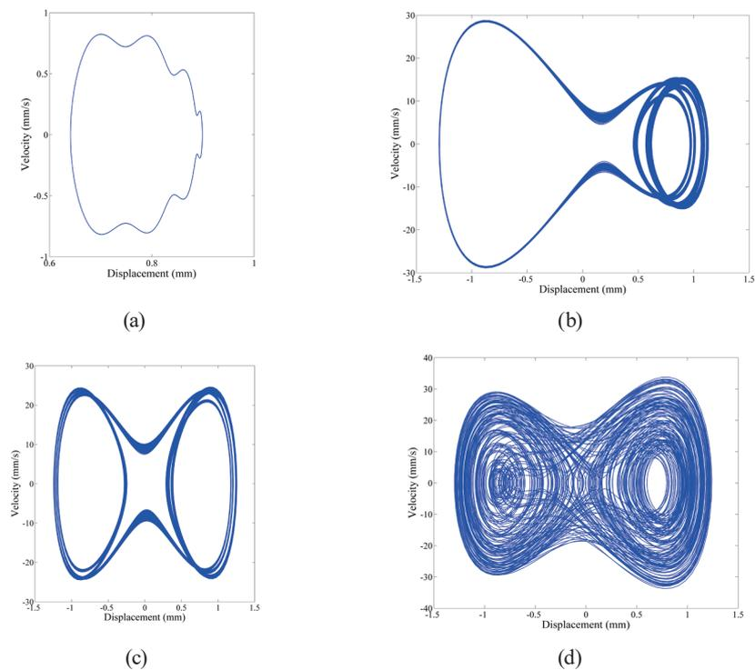
Fig. 10. (Color online) Phase diagram of the diamagnetic levitation structure under the excitation frequency of 1 Hz and different amplitudes of (a) 4, (b) 7.5, (c) 8.1, and (d) 8.1 mm.
