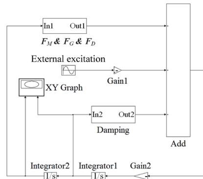
Fig. 8. Simulink model for the diamagnetic levitation structure.
