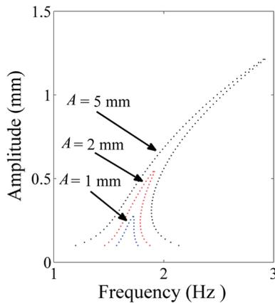
Fig. 7. (Color online) Amplitude–frequency response of the diamagnetic levitation structure.
