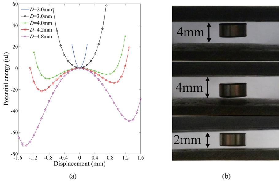
Fig. 4. (Color online) Bistable state of the diamagnetic levitation structure: (a) potential energy curve of floating and (b) equilibrium states.
