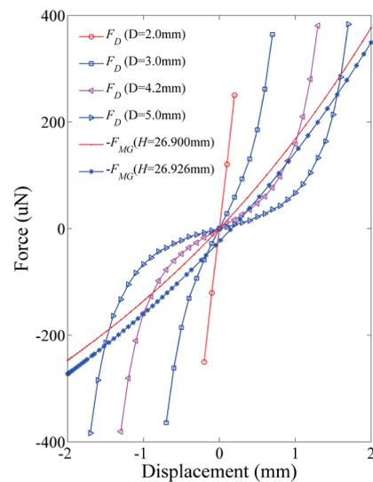
Fig. 3. (Color online) Force curve of the floating magnet.
