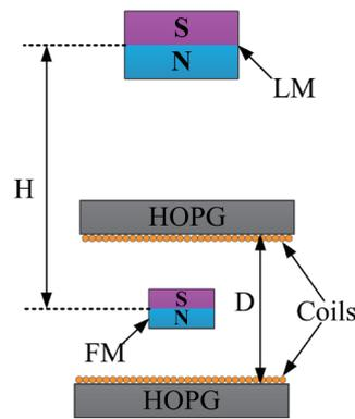
Fig. 1. (Color online) Schematic of vibration energy harvester.
