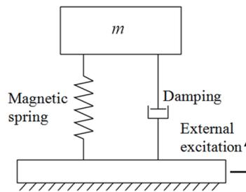
Fig. 6. Equivalent spring–mass model.
