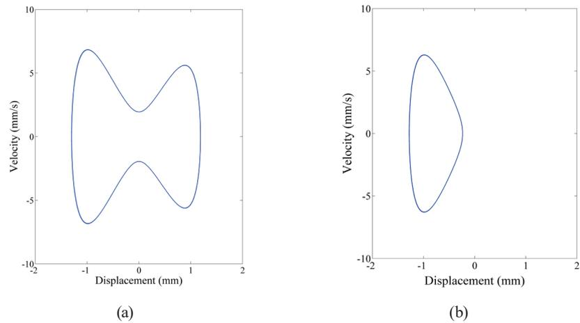
Fig. 9. (Color online) Phase diagram of free vibration: (a) asymmetrical and (b) symmetrical structures.
