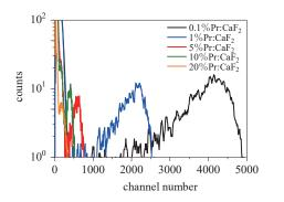
Fig. 5. (Color online) Pulse height spectra of  $Pr:CaF_2$  crystals under  $\alpha$ -ray irradiation.
