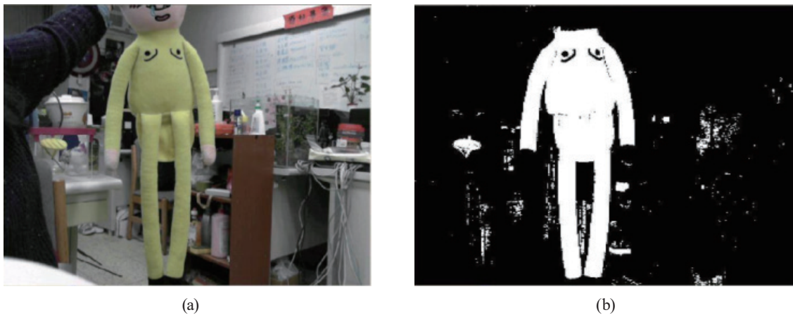
Fig. 7. (Color online) (a) RGB image and (b) binarized image (with speckle noises).
