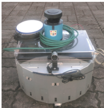
Fig. 1. (Color online) WMR with laser sensor, DGPS system, web camera and notebook.
