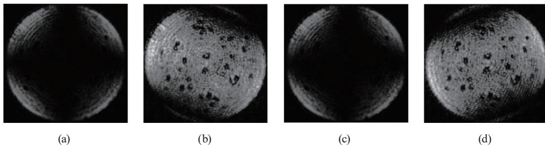
Fig. 4. Rotation of the azimuthal angle of QWP Q<sub>1</sub>. (a) 0, (b) 45, (c) 90, and (d) 135°.
