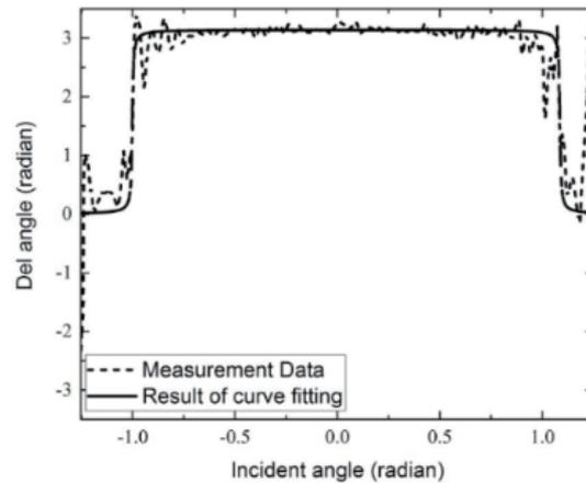
Fig. 8. Delta angle of SiO<sub>2</sub>.
