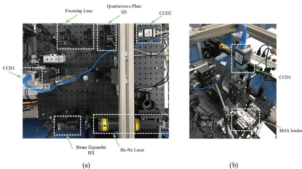
Fig. 3. (Color online) Optical system for flying height measurements. (a) Full diagram of micro-ellipsometer. (b) HGA loader.
