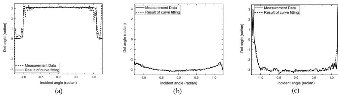
Fig. 12. Delta angles of (a) SiO<sub>2</sub>, (b) Au, and (c) AlTiC.
