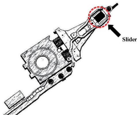
Fig. 1. (Color online) Example of a slider installed on an HGA.<sup>(1)</sup>
