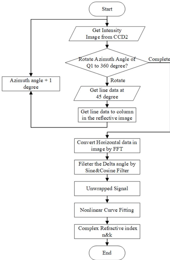
Fig. 5. Procedure of optical image processing.
