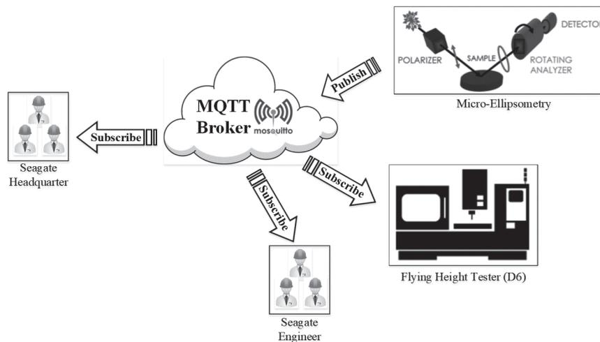
Fig. 9. Private cloud structure of optical characterization.
