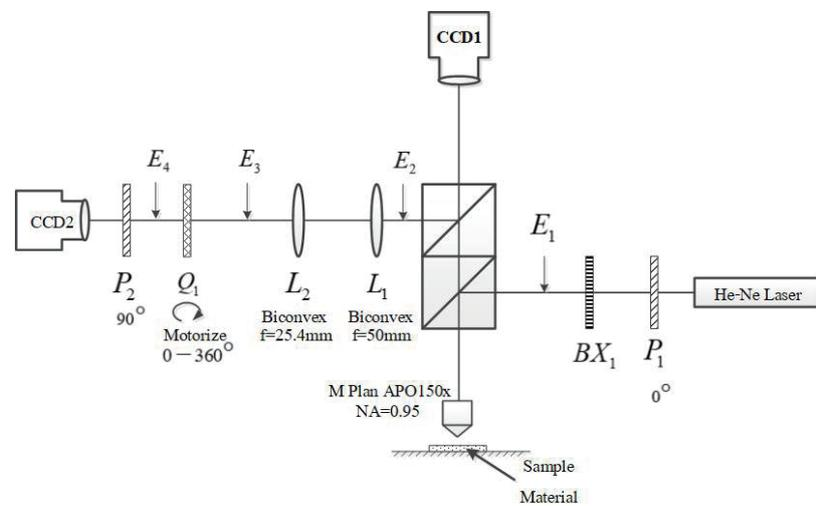
Fig. 2. Diagram of back focal plane micro-ellipsometer.
