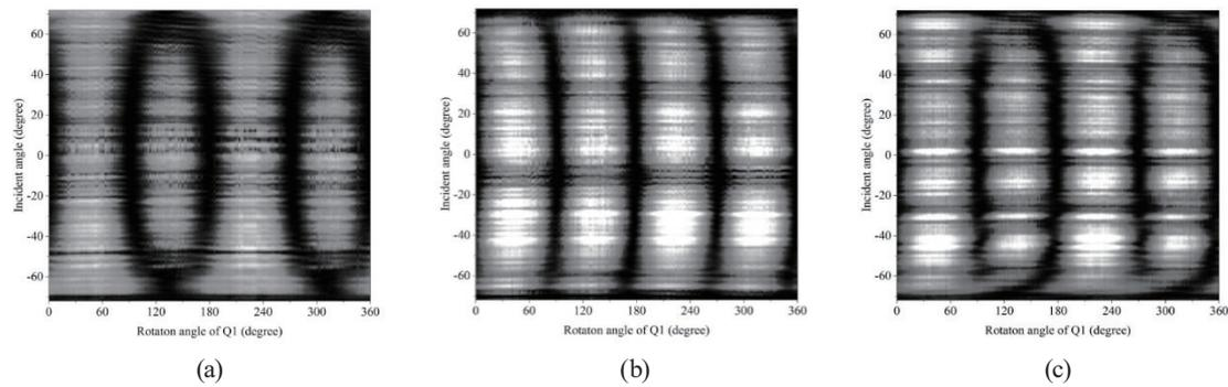
Fig. 11. Stack intensity images of (a) SiO<sub>2</sub>, (b) Au, and (c) AlTiC.
