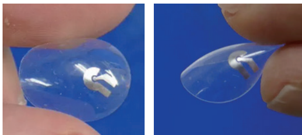
Fig. 2. (Color online) Photographs of SCL biosensor showing flexibility of not only the lens but also the coated electrodes.
