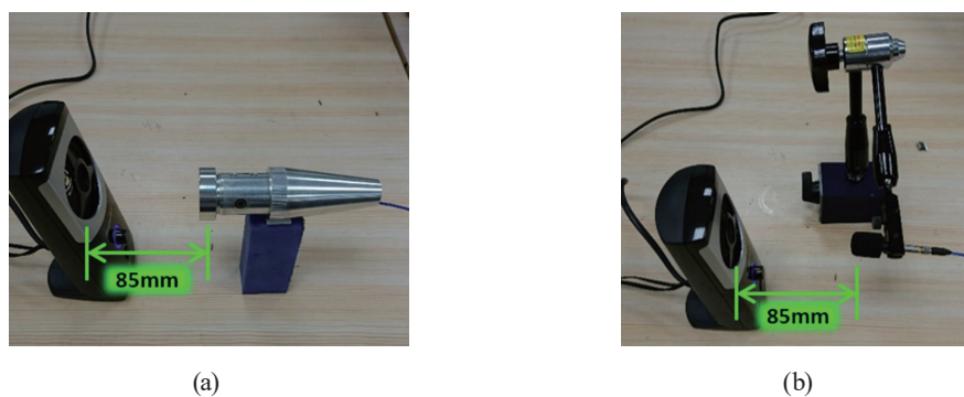
Fig. 5. (Color online) Positions of speaker and microphone: (b) with and (a) without waterproof device.
