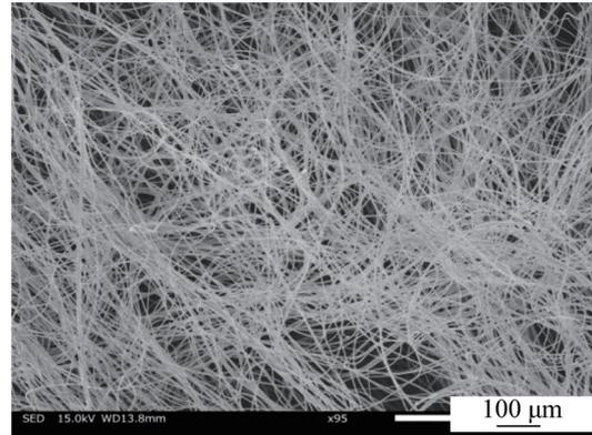
Fig. 11. SEM image of PP microfibers melt spun from the  $\varnothing 40 \mu\text{m}$  spinning nozzle in Fig. 7. (Duration: 15 min, electric power: 800 W)
