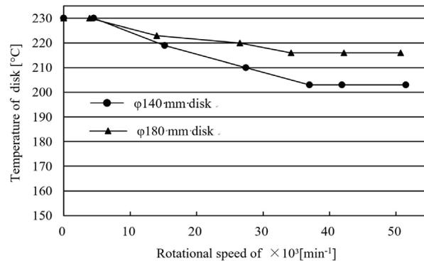
Fig. 9. Relationship between rotation speed/frequency of the disk and temperature of the disk (gap: 2 mm).
