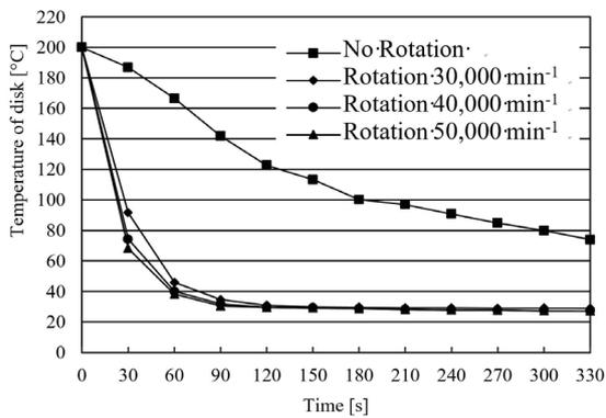
Fig. 10. Relationship between rotation time and temperature of disk (gap: 2 mm).
