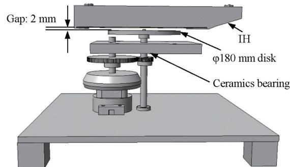
Fig. 7. Whole view of the present spinning equipment with IH.
