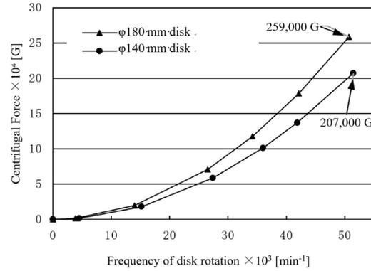
Fig. 6. Rotation speed/frequency  $\omega$  of the disk and centrifugal force.
