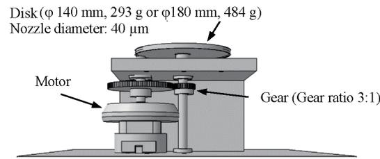
Fig. 1. Overview of fiber-spinning equipment (weight: 20 kgf).
