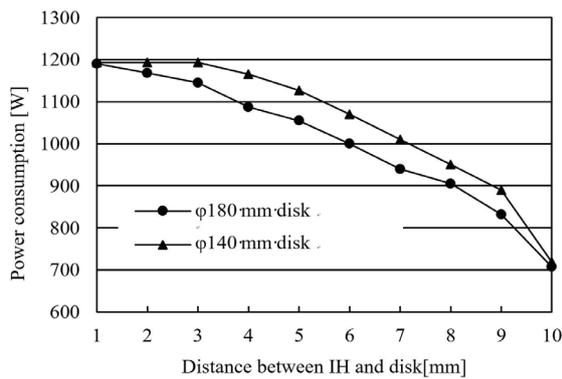
Fig. 8. Relationship of distance/gap between IH and disk with power consumption.
