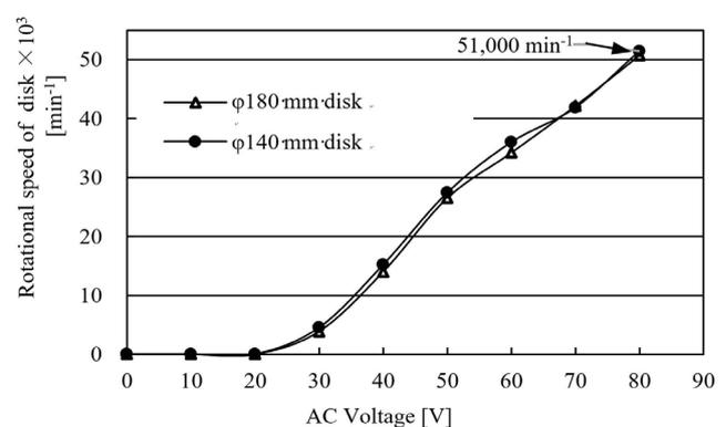
Fig. 4. Input voltage and rotation speed of the disk.
