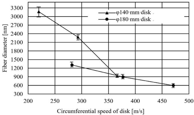
Fig. 14. Circumferential disk speed vs fiber diameter.
