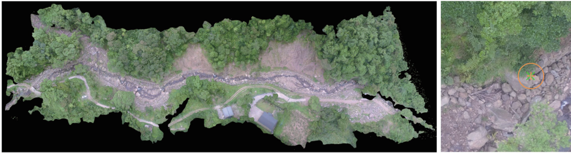
Fig. 12. (Color online) 3D model obtained after point cloud densification.
