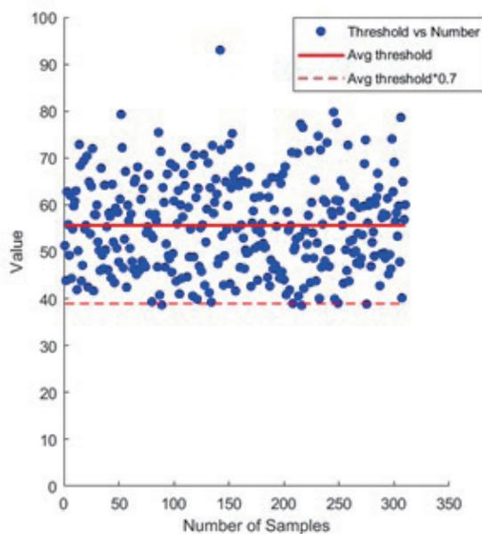
Fig. 6. (Color online) Threshold value distribution plotted by the difference value of maximum and minimum pitch angles of every step count.
