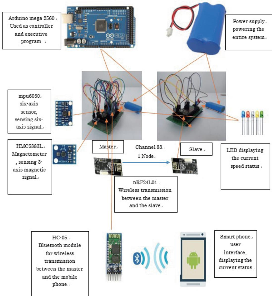
Fig. 2. (Color online) Apparatus for gait speed feature with dual wireless communication on right and left feet.
