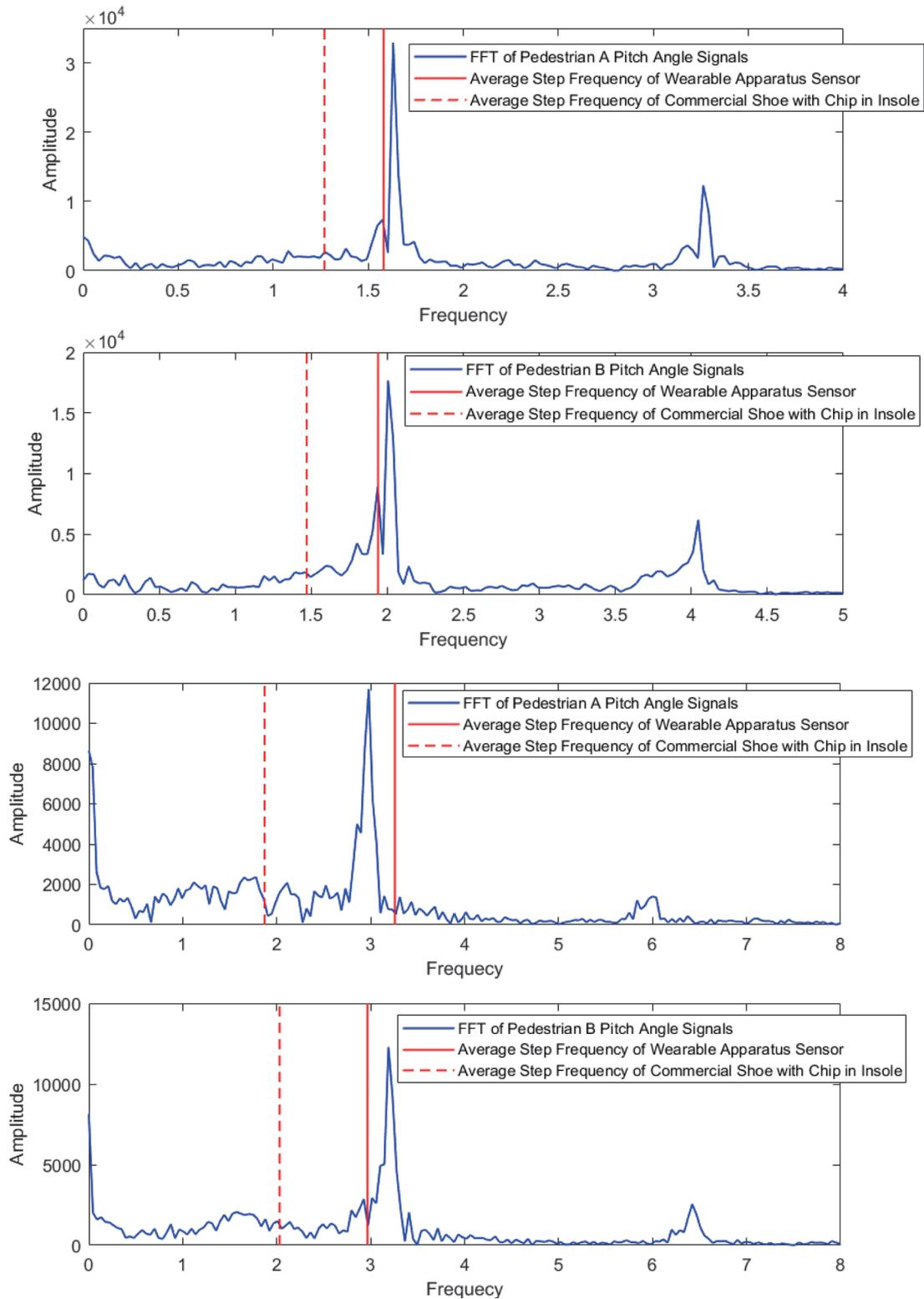
Fig. 10. (Color online) Frequency response calculation by FFT (signal in blue color) of the pitch angle history, the commercial shoe with chip in insole (dashed line in red), and the calculated step frequency (solid line in red) under the treadmill speeds of 4 km/h (left) and 8 km/h (right) for pedestrians A and B.
