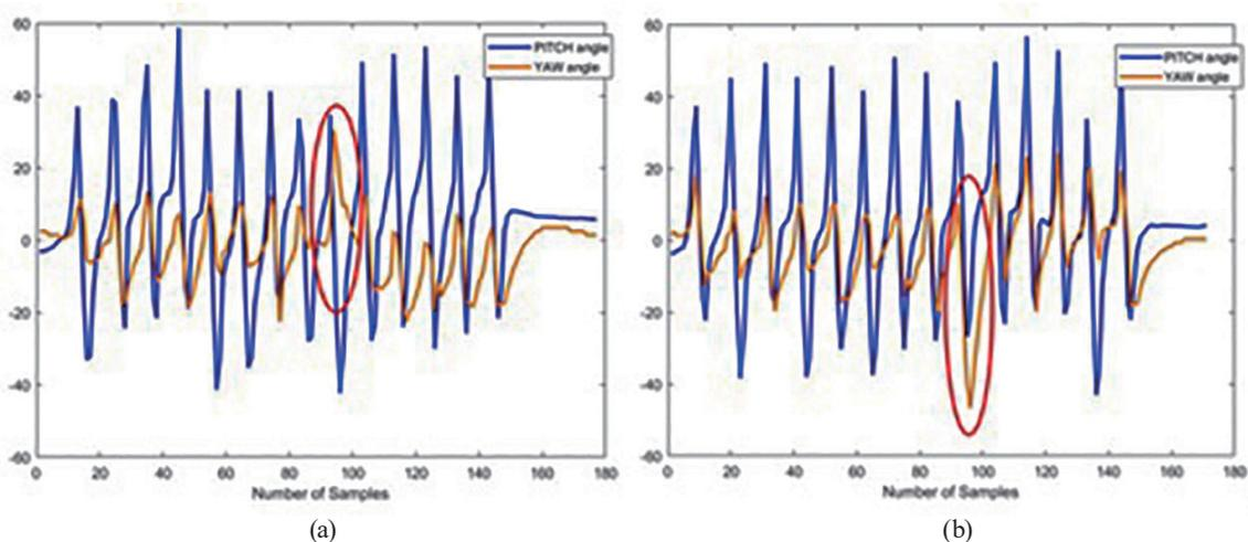
Fig. 8. (Color online) (a) Left turn and (b) right turn signals of the pitch and yaw angles.
