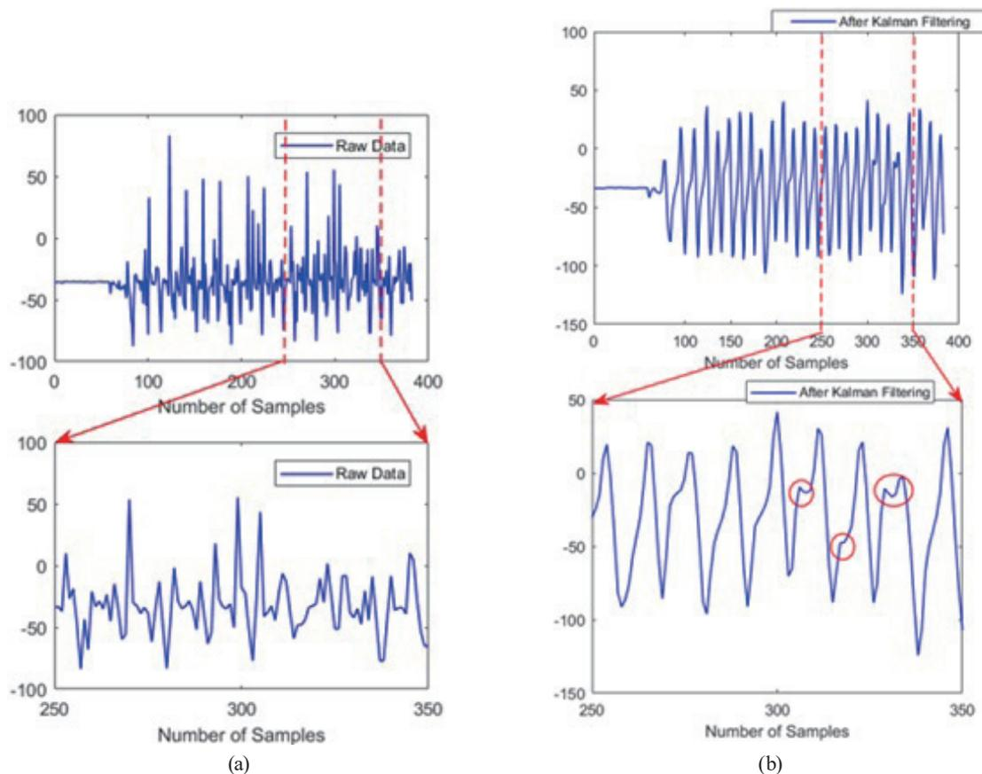
Fig. 4. (Color online) (a) Raw Euler pitch angle data before KF. (b) Calculated swing pitch angle signal after KF.
