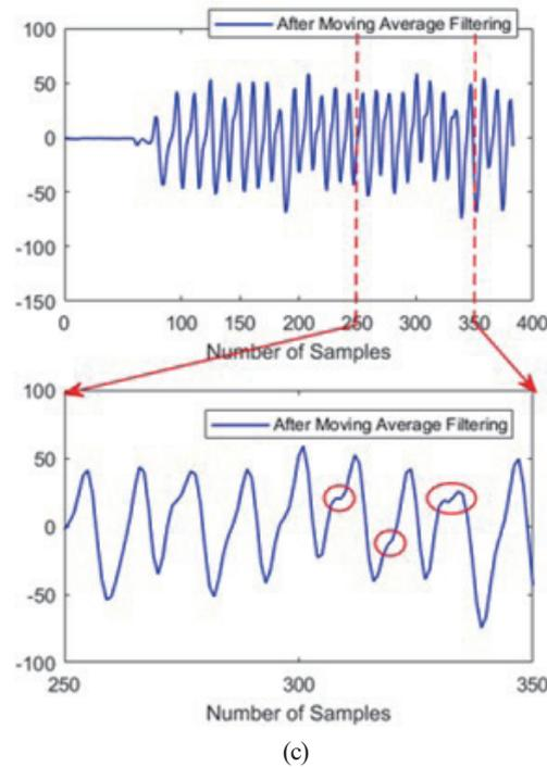
Fig. 4. (continued) (c) Calculated pitch angle by applying moving average right after KF in Fig. 4(b).
