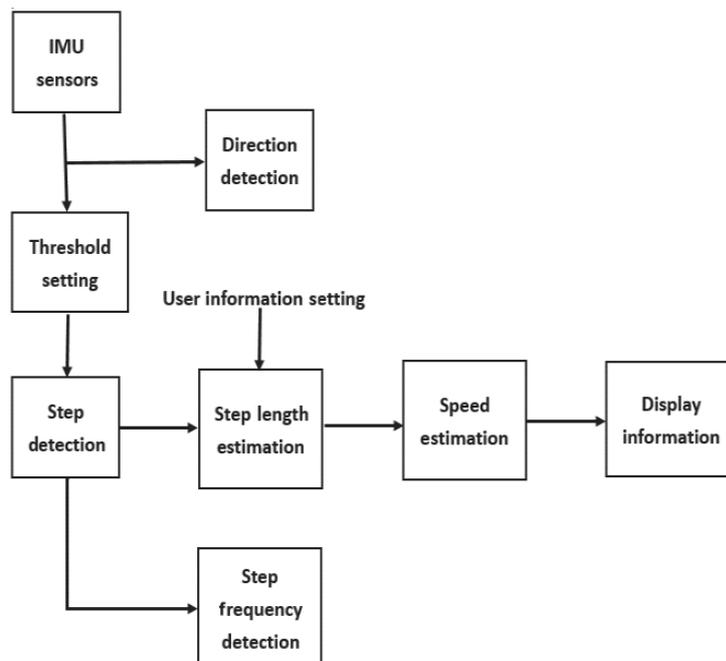
Fig. 1. Flow chart of step count, heading, and speed by using a single IMU.
