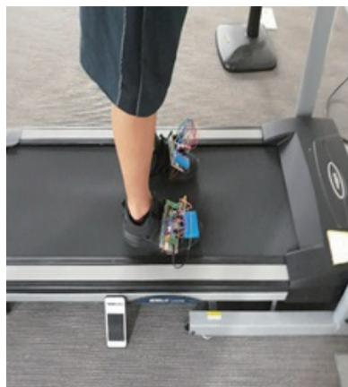
Fig. 9. (Color online) Testing the developed apparatus with a treadmill and commercial shoes with chip in insole.
