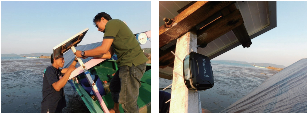
Fig. 1. (Color online) GPS tracker installation on small boat.
