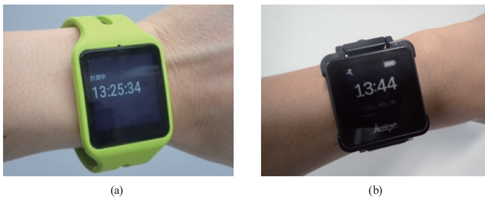
Fig. 2. (Color online) Wearable devices used in this study. (a) SmartWatch 3 SWR 50 (Sony Mobile Communications Inc.) and (b) ActiGraph GT9X Link (ActiGraph LLC).
