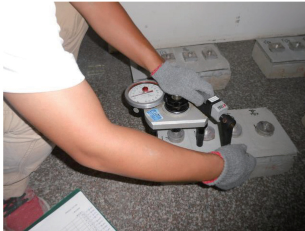
Fig. 5. (Color online) Tile pullout experiment.
