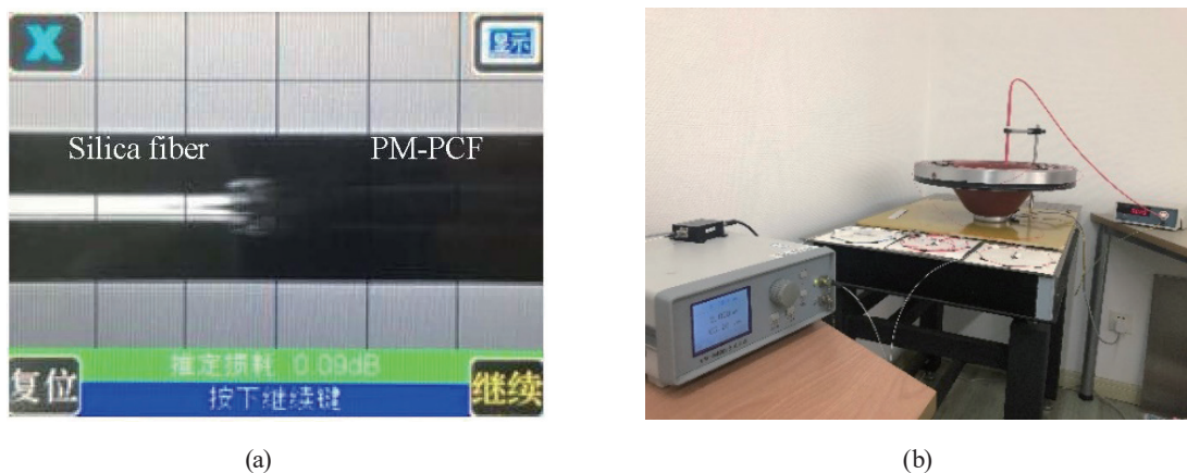
Fig. 6. (Color online) Images of (a) the fusion of two fibers and (b) the platform.
