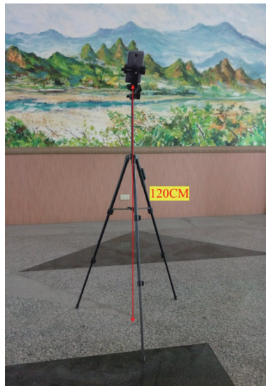
Fig. 21. (Color online) The mobile device is placed on a tripod at 120 cm above ground.
