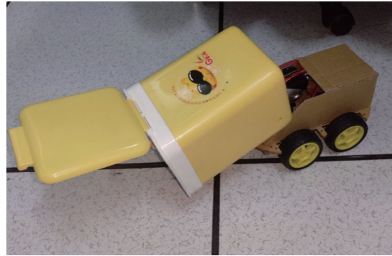
Fig. 9. (Color online) The trash can tilts to dump the trash.
