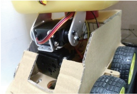
Fig. 8. (Color online) Servo motor for tilting the trash can.
