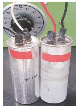
Fig. 2. (Color online) Aged power capacitors.
