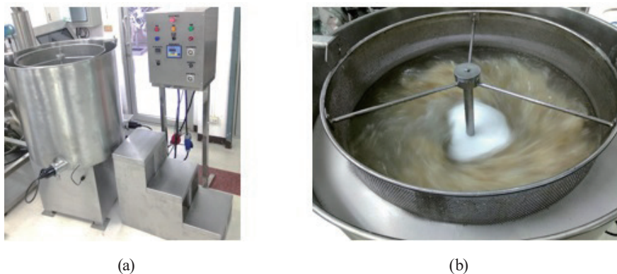
Fig. 6. (Color online) (a) Desalting machine. (b) Running in the centrifugal mode.
