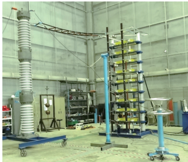
Fig. 16. (Color online) Arrangement of LIV withstand test.
