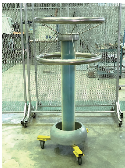
Fig. 10. (Color online) Developed saline solution voltage divider with grading rings.
