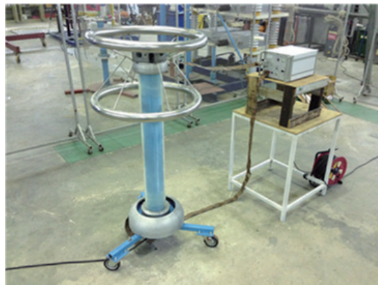
Fig. 13. (Color online) Experimental setup for unit step response test.
