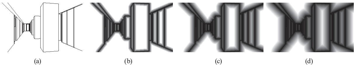
Fig. 6. Examples of gradient dilation images: (a) q_w = 0 , (b) q_w = 10 , (c) q_w = 20 , and (d) q_w = 30 .
