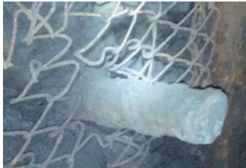
Fig. 1. (Color online) Actual scene of drill rod sticking in underground coal mine.
