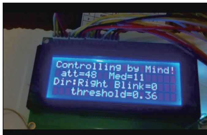
Fig. 7. (Color online) Output data of the SMWCW displayed on the LCD screen.
