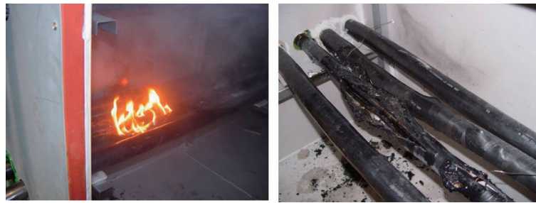
Fig. 7. (Color online) Cable ignition inside the prototype owing to overcurrent (1st experiment).
