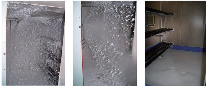
Fig. 10. (Color online) Foam discharge inside the experimental space (without ignition, 2nd experiment).
