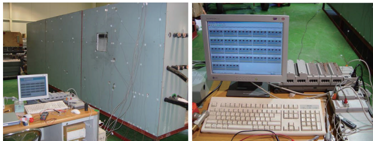
Fig. 5. (Color online) Thermocouple and data acquisition system for temperature measurement in prototype equipment.
