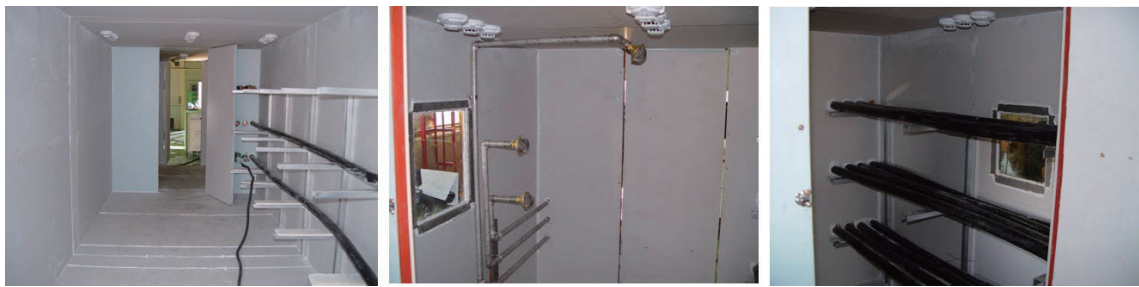
Fig. 3. (Color online) Form head and cable layout inside the prototype experimental equipment.
