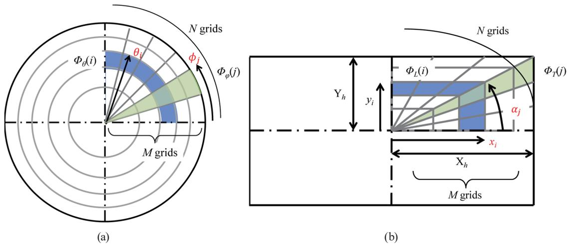
Fig. 1. (Color online) Schematic illustration showing luminous flux mapping relationship between (a) light source and (b) target plane.
