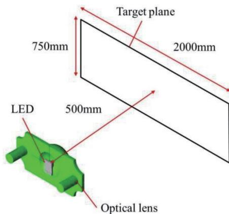
Fig. 2. (Color online) Schematic illustration of LED illumination device and illumination requirement.
