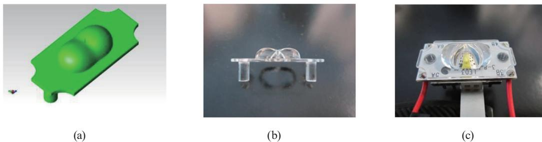
Fig. 7. (Color online) (a) Computer-generated model of optical lens, (b) prototype of TGM-designed LED free-form lens, and (c) LED illumination device.
