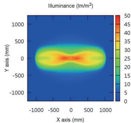
Fig. 3. (Color online) Simulation results showing non-uniform illuminance distribution when TGM method is not applied.
