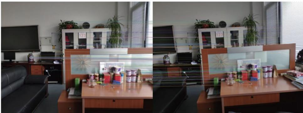
Fig. 8. (Color online) Mismatch elimination using RANSAC algorithm.
