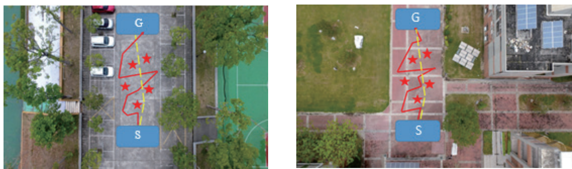
(a) (b) Fig. 6. (Color) Two test environments. The obstacles are marked in red. The shortest path is the yellow one and the planned path is the red one. (a) Parking area with smooth road. (b) Trail.
