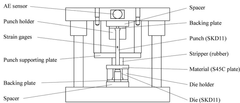
Fig. 1. Punching device with function for measuring axial stress of punch and AE signal.
