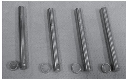
Fig. 11. Fractured punches.
