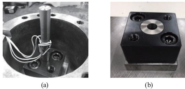
Fig. 2. Photos of punching tools. (a) Punch with strain gages. (b) Die mounted on holder.
