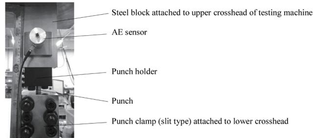
Fig. 8. Tensile test of punch.
