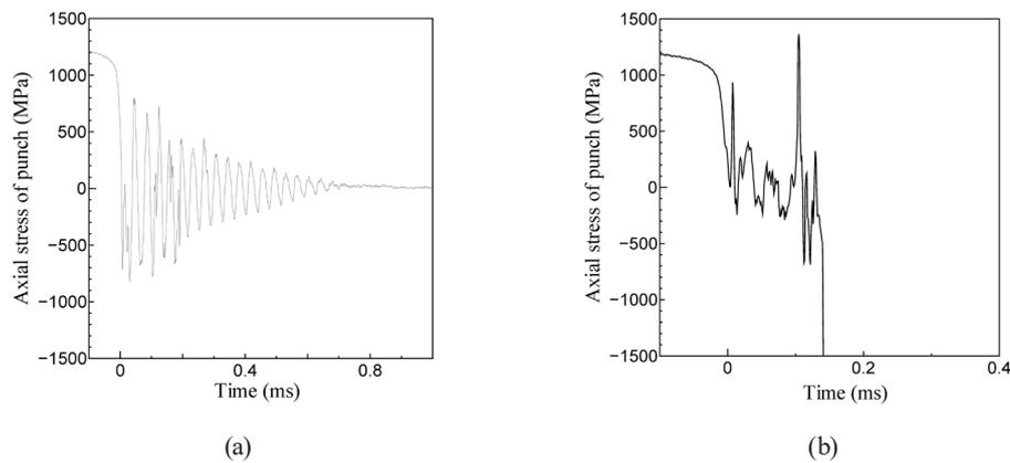
Fig. 6. Axial stress of punch (thickness: 6 mm,  $R$ : 0.30 mm). (a) First punching and (b) second punching.
