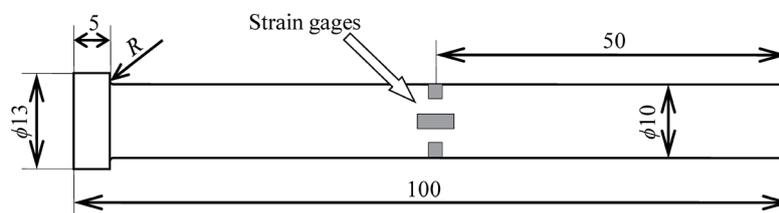
Fig. 3. Dimensions of stepped circular punch and attachment position of strain gages.
