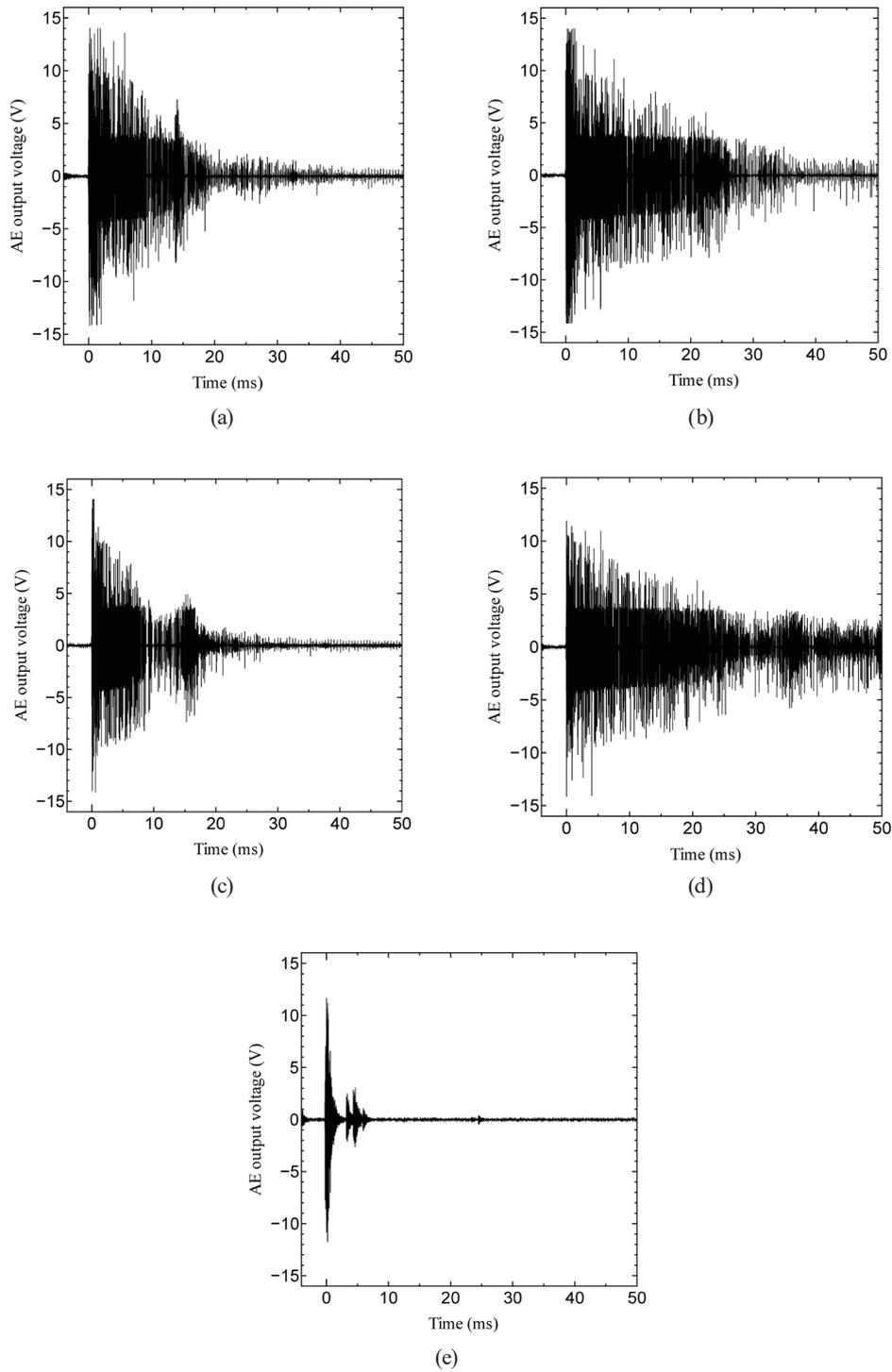
Fig. 13. AE waveform for punch fillet radius  $R$  of 0.32 mm. (a) First punching (thickness: 5 mm), (b) second punching (6 mm), (c) third punching (5 mm), (d) fourth punching (6 mm), and (e) fifth punching (5 mm).
