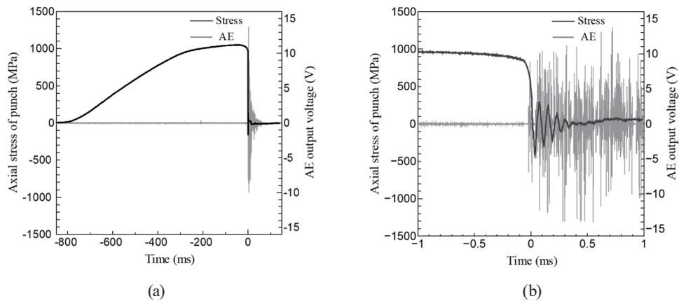
Fig. 5. Axial stress of punch and AE signal during punching (thickness: 5 mm). (a) Variation during punching and (b) variation before and after material fracture.
