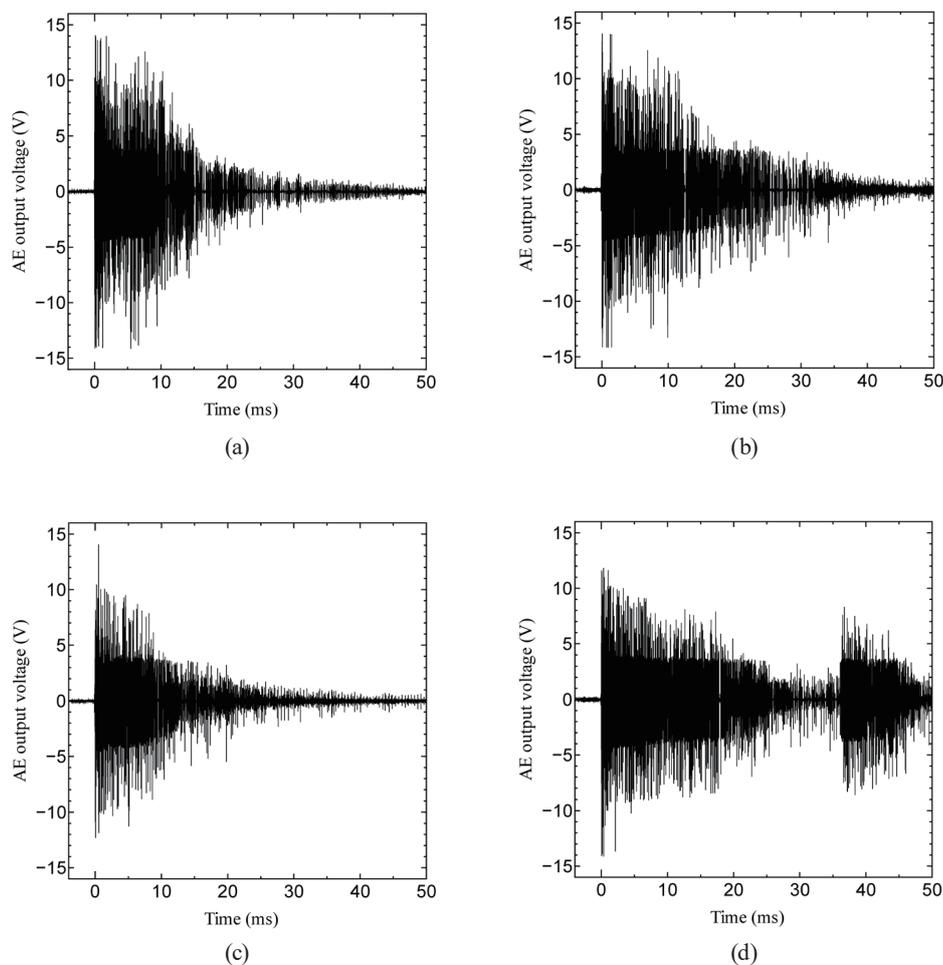
Fig. 12. AE waveform for punch fillet radius  $R$  of 0.39 mm. (a) First punching (thickness: 5 mm), (b) second punching (6 mm), (c) third punching (5 mm), and (d) fourth punching (6 mm).
