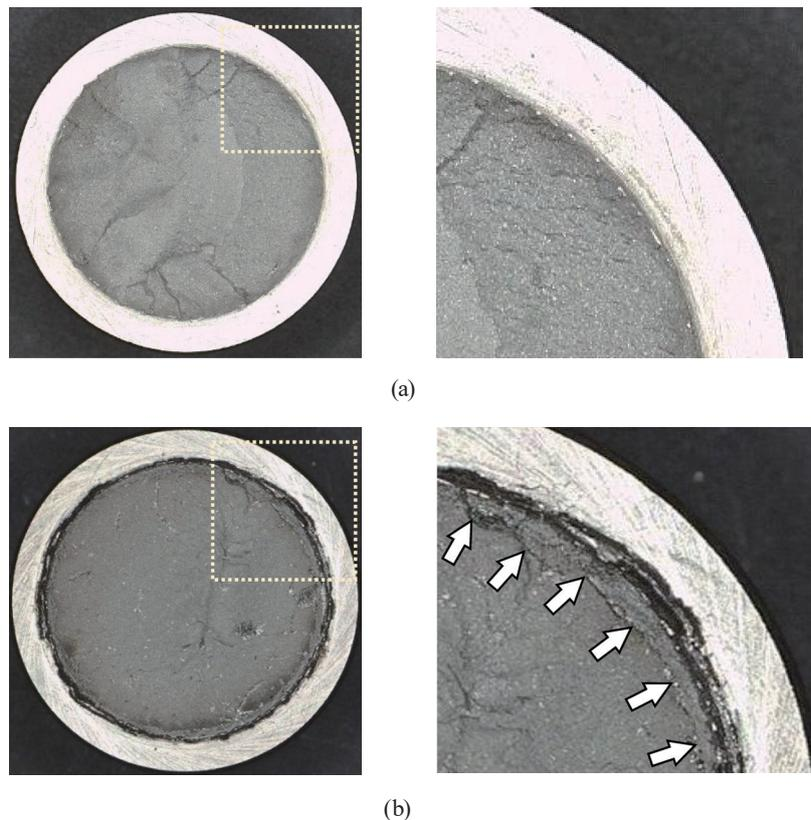
Fig. 14. Appearance of fracture at stepped portion of punch. (a) (left) General view of fractured surface and (right) magnified view of rectangular area in left photo;  $R = 0.39$  mm. (b) (left) General view of fractured surface and (right) magnified view of trace of small crack at fourth punching;  $R = 0.32$  mm.
