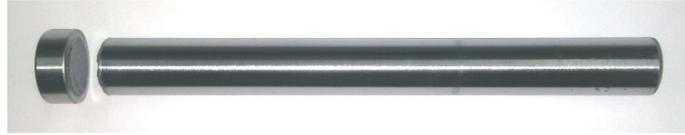
Fig. 7. Fracture of stepped circular punch.
