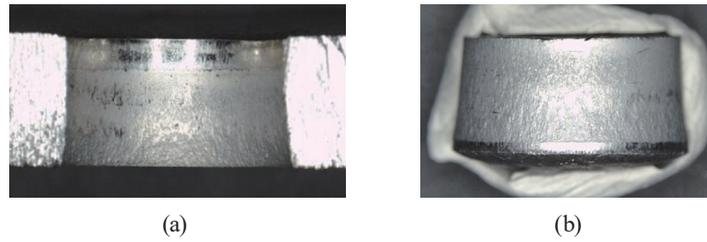
Fig. 4. Cross sections of (a) hole and (b) scrap (nominal thickness: 6 mm).
