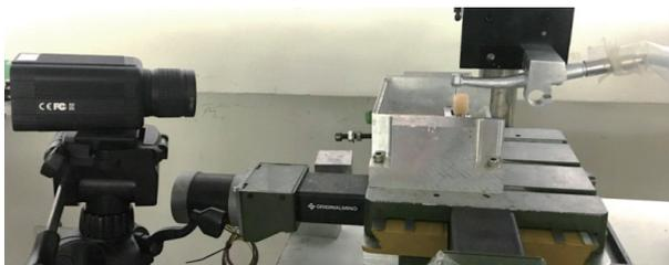
Fig. 10. (Color online) Experimental setup for thermal imaging during cutting.
