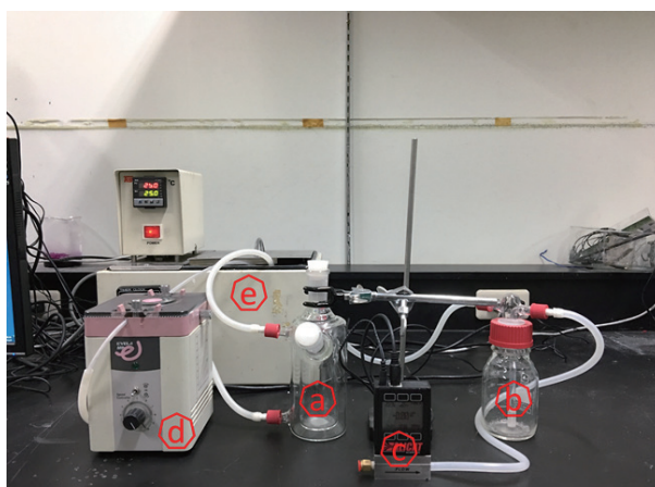
Fig. 4. (Color online) Experimental setup for evaluating hydrogen production efficiency: (a) hydrogen production container, (b) gas filter flask, (c) hydrogen mass sensor, (d) catalyst bed flow pump, and (e) catalyst bed constant temperature water tank.
