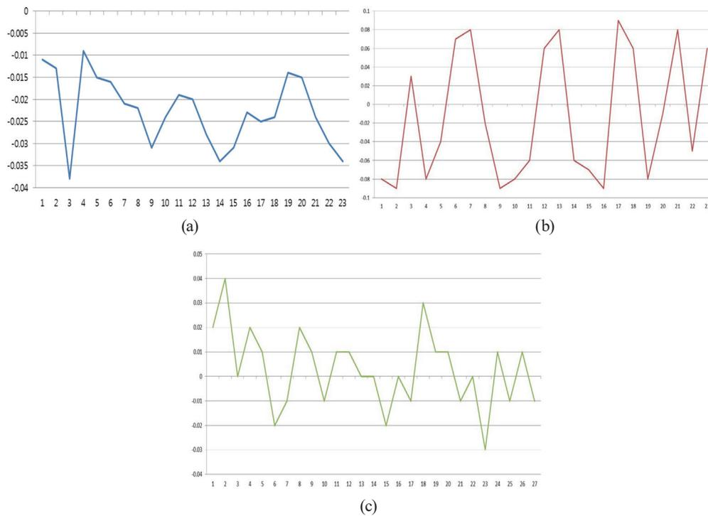
Fig. 18. (Color online) Deviation of values measured using scanner. (a) DBH. (b) Tree height. (c) Diameter of felled tree.
