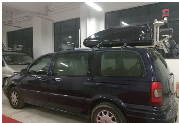
Fig. 7. (Color online) Newly developed vehicle and mobile measurement system. The mobile measurement system is composed of laser scanners, the GNSS global positioning system, the IMU inertial navigation sensor, an odometer, a panoramic camera, and other sensor elements.
