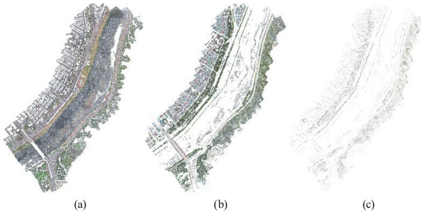
Fig. 9. (Color online) (a) Ground, (b) buildings, and (c) high-density vegetation classified using GlobalMapper.
