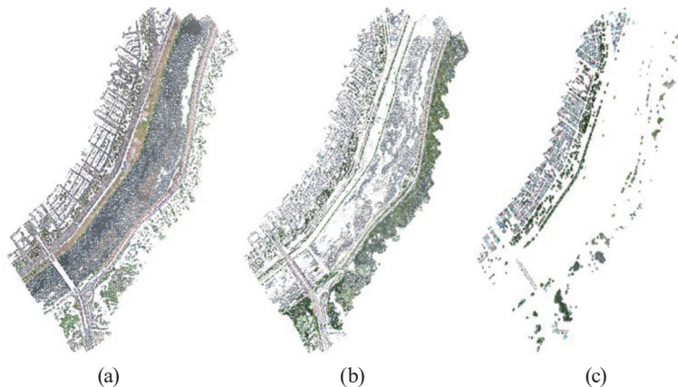
Fig. 10. (Color online) (a) Ground, (b) high-density vegetation, and (c) buildings classified using Inpho.
