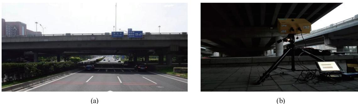
Fig. 6. (Color online) Fengbei Bridge and IBIS-S layout. (a) Fengbei Bridge and (b) dynamic deflection measurement of Fengbei Bridge using IBIS-S.
