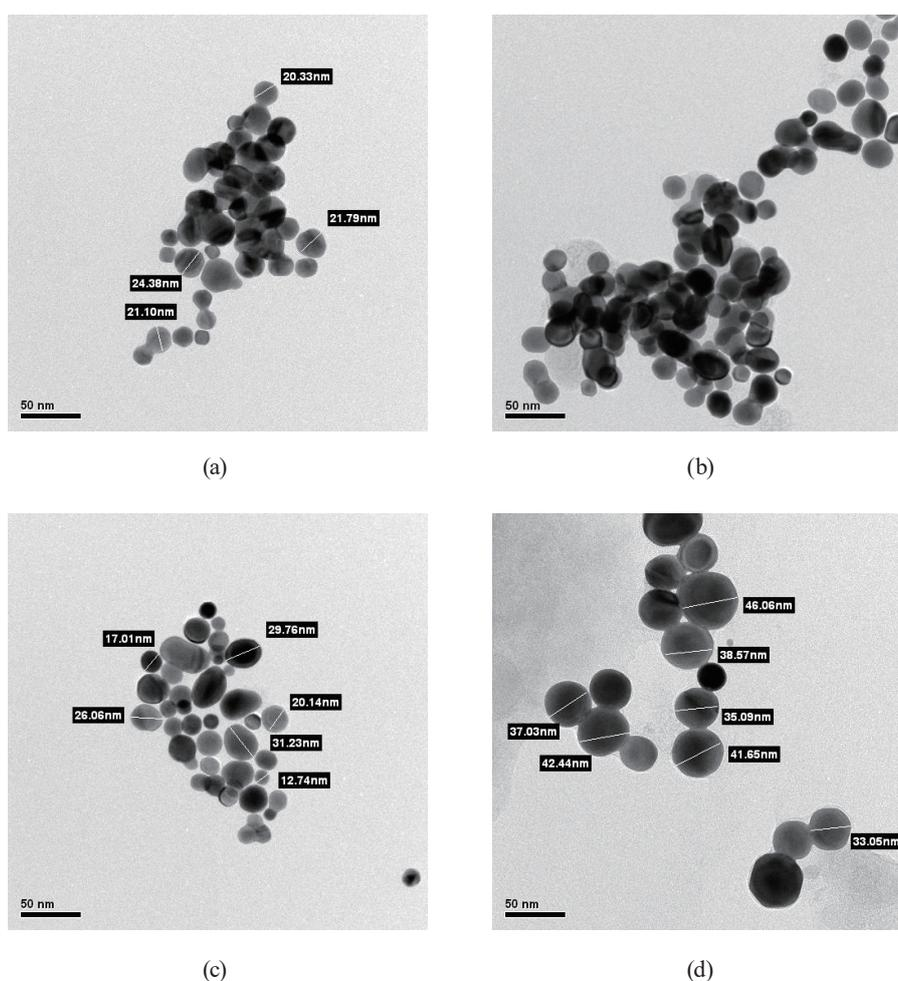
Fig. 5. TEM images of GNPs in condensation reaction obtained with (a) 30, (b) 50, (c) 70, and (d) 90  $\mu\text{l}$  of NaOH added to growth solution.
