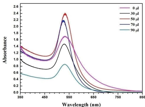
Fig. 4. (Color online) Light absorbance spectra of GNP solutions obtained by condensation reaction with different amounts of NaOH added to growth solution.
