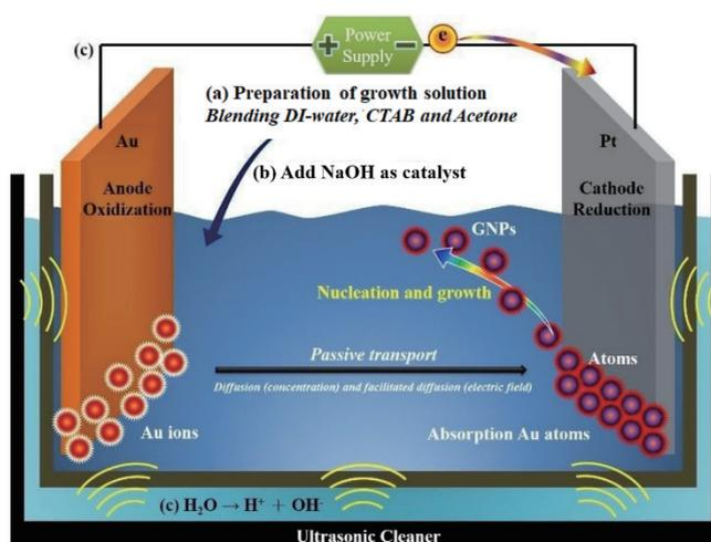
Fig. 1. (Color online) Schematic diagram of GNP preparation via electrochemistry: (a) prepare growth solution, (b) add NaOH as catalyst to form micelle template for condensation reaction, and (c) perform continuous electrolysis and oscillation.
