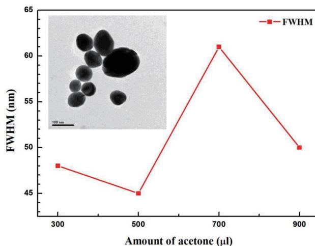
Fig. 3. (Color online) FWHM calculated from absorbance of GNP solutions with various amounts of added acetone. The inset shows a TEM image of GNPs added with 500  $\mu\text{l}$  of acetone.
