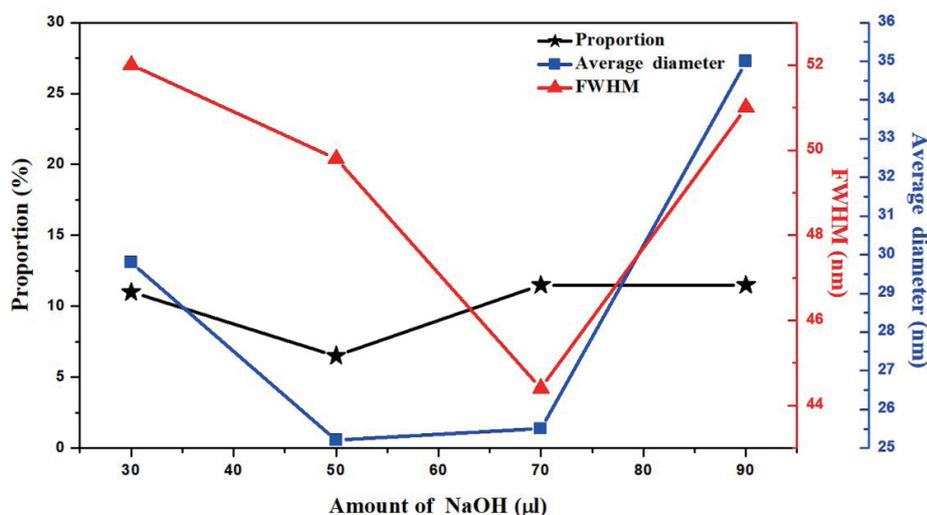
Fig. 6. (Color online) Calculated proportion of black area in images (stars), FWHM (triangles), and average diameter (squares) of GNPs obtained with 30, 50, 70, and 90  $\mu\text{l}$  of NaOH added to growth solution.
