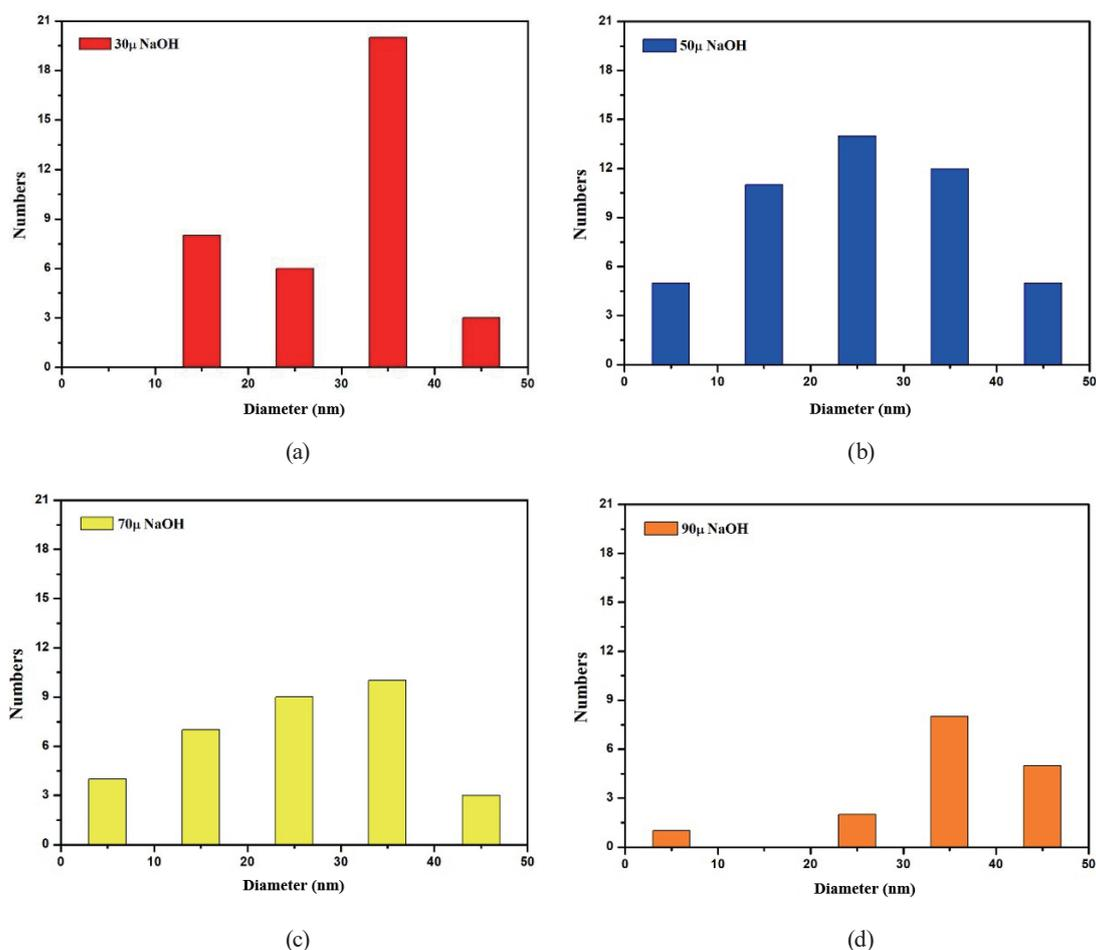
Fig. 7. (Color online) Histograms showing size distributions of GNPs obtained with 30, 50, 70 and 90  $\mu\text{L}$  of NaOH added to growth solution.
