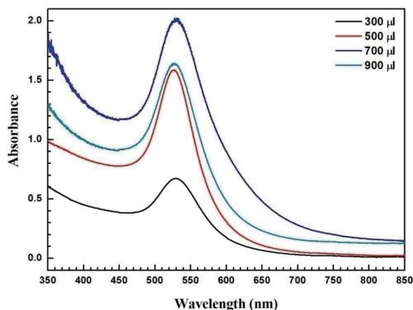
Fig. 2. (Color online) Light absorbance spectra of GNPs synthesized in growth solution with various amounts of added acetone.
