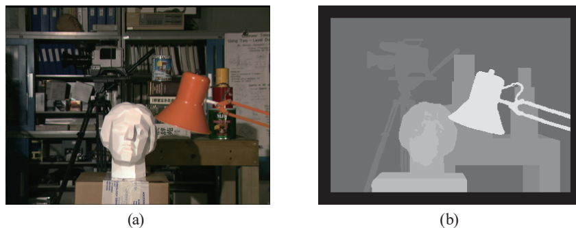
Fig. 1. (Color online) Depth image. (a) Original image and (b) depth image demonstrating optical parallax.
