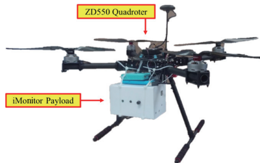
Fig. 5. (Color online) UAV (ZD550) equipped with iMonitor box payload.
