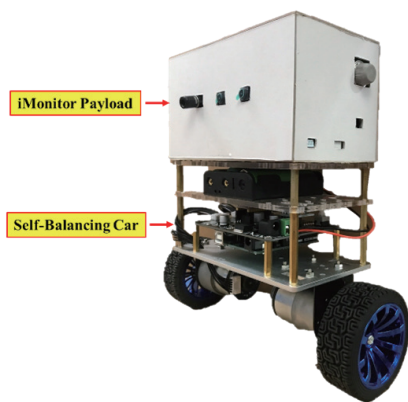
Fig. 4. (Color online) UGV (self-balancing car) equipped with iMonitor payload.
