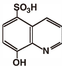
Fig. 2. Structural formula of the 8-Hydroxyquinoline-5-sulphonic acid reagent for cadmium ions. The OH group of SO 2 OH is attached to the glass film. The OH group adjacent to nitrogen N and the nitrogen atom form a bidentate chelating complex with cadmium.
