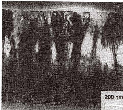
Fig. 6. TEM micrograph of an arsenic-doped polycrystalline layer, stress annealed at 1000°C for 80 s.
