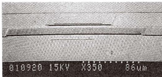
Fig. 2. Straight free-standing bridge, fabricated using RTA stress-annealed silicon.
