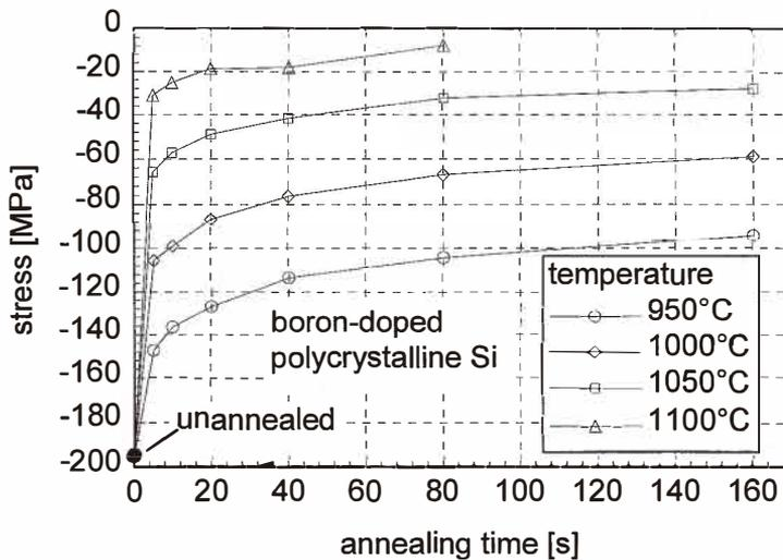
Fig. 3. Stress relaxation characteristics for a 1- $\mu\text{m}$ -thick boron-doped polycrystalline silicon layer annealed by RTA.
