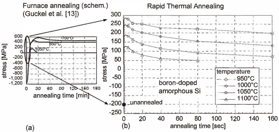
Fig. 5. (a) Annealing curves for amorphous silicon during furnace annealing (Guckel *et al.*<sup>(13)</sup>). (b) Stress relaxation of boron-doped amorphous silicon annealed by RTA.
