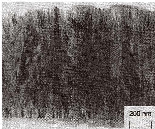
Fig. 7. TEM micrograph of an unannealed polycrystalline silicon layer.
