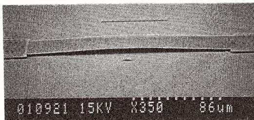
Fig. 1. Buckled bridge, fabricated using as-deposited polycrystalline silicon.
