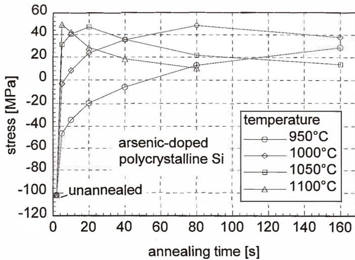
Fig. 4. Stress relaxation curves for a 1- $\mu\text{m}$ -thick arsenic-doped polycrystalline silicon layer annealed by RTA.
