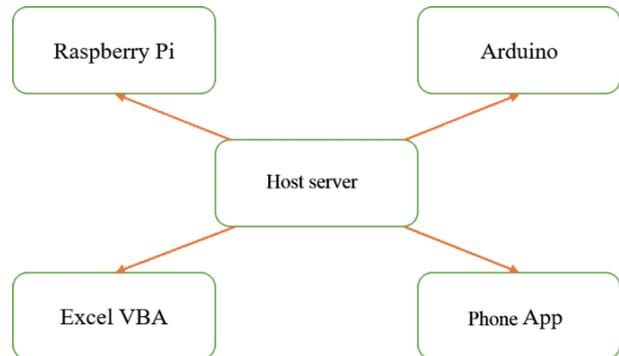
Fig. 9. (Color online) Architecture of powered wheelchair data monitoring system.
