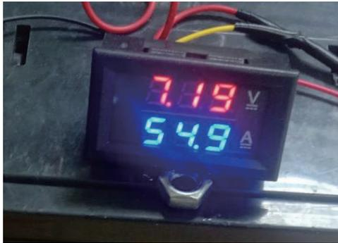
Fig. 4. (Color online) DC100 V LED DC dual-display digital voltmeter.
