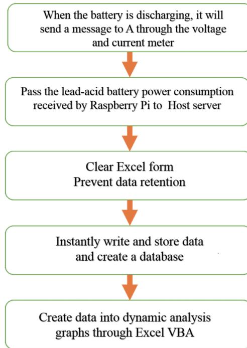
Fig. 16. (Color online) Flowchart for monitoring lead-acid battery power consumption.
