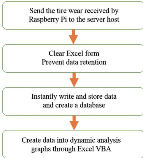
Fig. 13. (Color online) Flowchart for monitoring tire wear.
